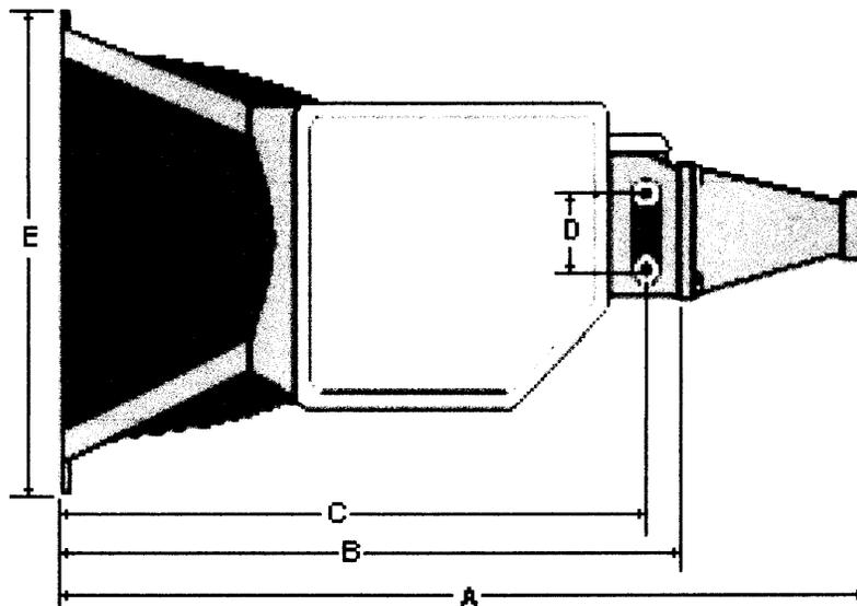
\*\*Dimension "C" is the distance from the bellhousing to the center of the transmission housing. The mount is usually part of the extension housing. The image shows it as part of the main housing. In reality, Dimension "C" is longer than Dimension "B".\*\*
